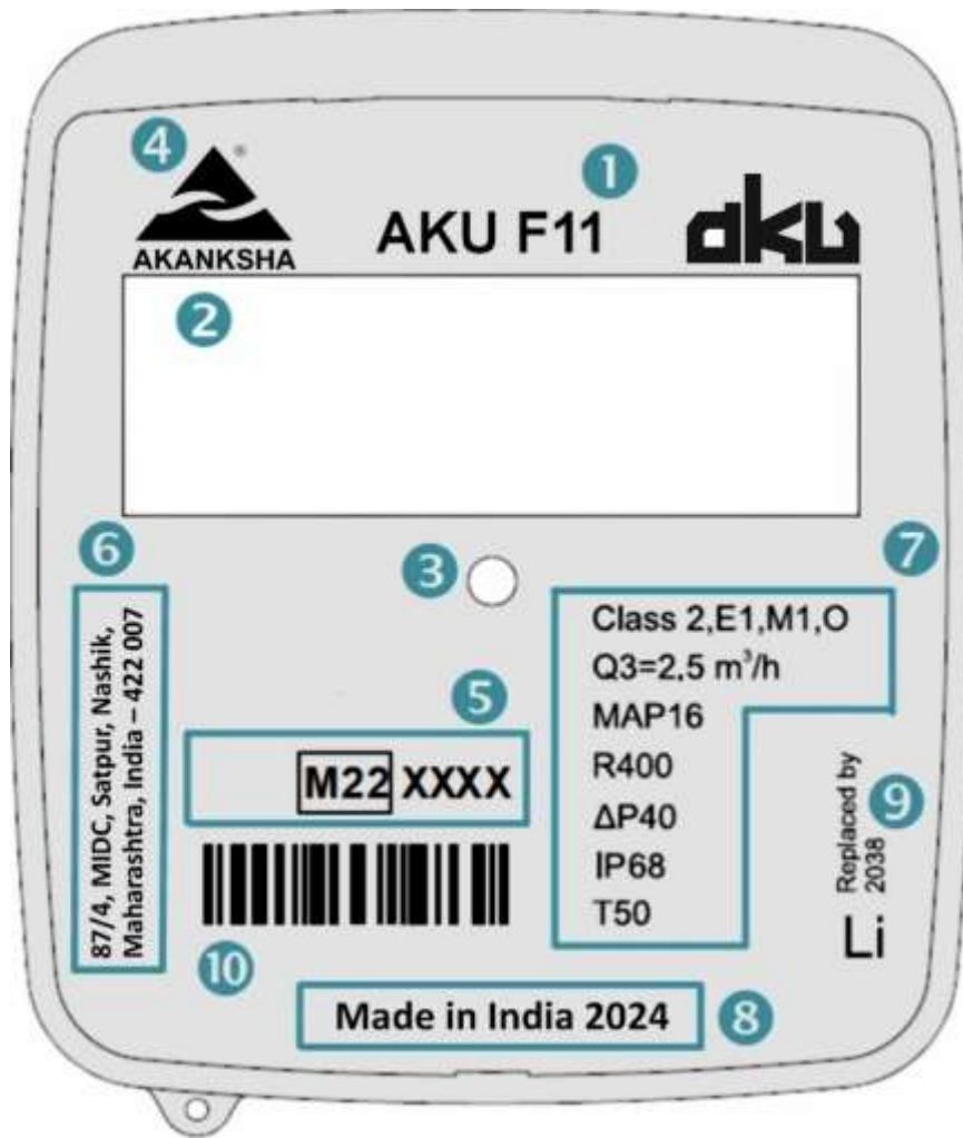
Fig.3. WM nameplate elements
